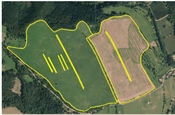
Fig. 2. Division of farmland blocks into smaller units at the site of Březová, Brumov-Bylnice. Linear contour plantings are arranged in a way minimising water erosion, at the same time allowing for continuation of large-scale tillage.
