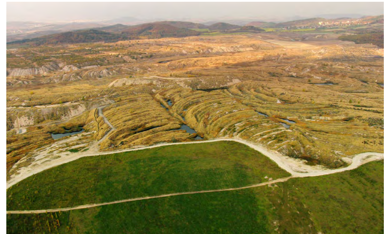
Fig. 6. In technical reclamations, the terrain is levelled, drained and prepared for cultivation by bringing on suitable topsoil. The upper part of this image of the Radovesice spoil bank shows an environment created by spontaneous succession, while the lower part shows the results of technical reclamation. (M. Hendrychová).
